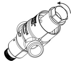
7. Remove the differential pressure regulator from the valve housing
