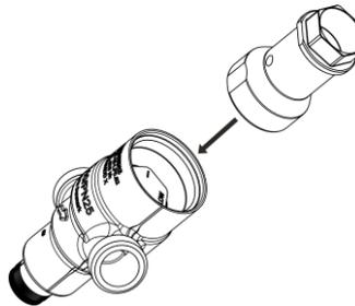
6. Loosen the differential pressure regulator
