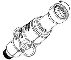
4. Remove the On/Off bonnet from the valve housing
