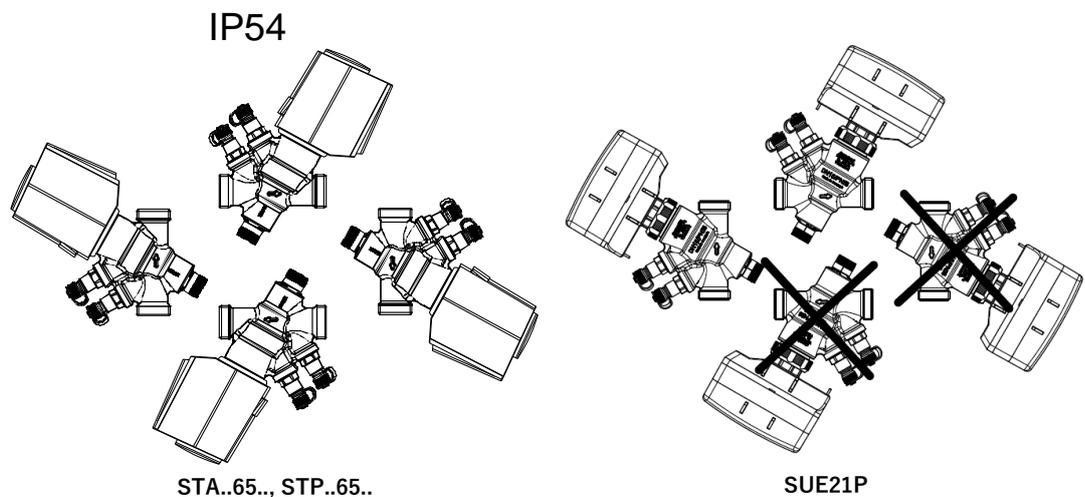
Thermal actuators STA..65.. and STP..65.. may be installed in any position.
