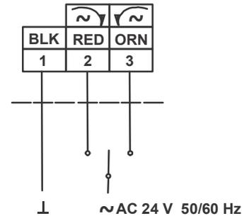
**Figure 2: VA9104-AGA-1S and VA9104-IGA-1S Control Wiring Diagram**
