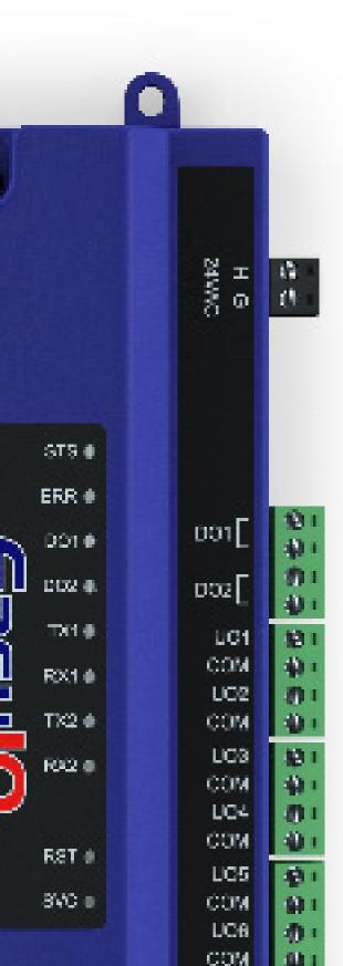
The FS-20 is a high performance server class controller with a 1.2 GHz quad core processor, 512 MB RAM and 8GB flash memory, powerful capabilities with HTML5 graphics and multifunctional adapter widgets. The built-in VPN client/server allows for secure remote connectivity, in line with your clients corporate policy, it is a unique feature for BMS controllers. The FS-20 supports IT standards, such as IPv6, 802.1x, MQTT and REST API.
