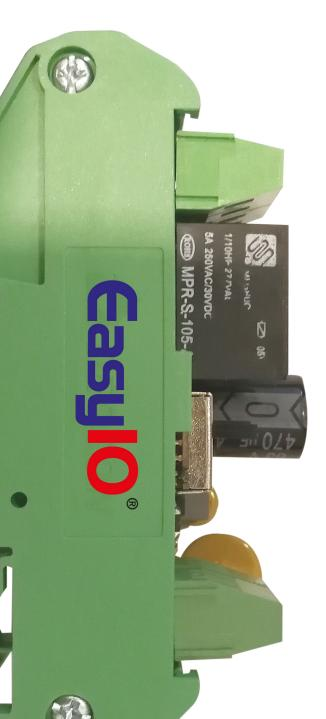
The FR-02 is a relay module which can be mounted on DIN rail. It allows 1 x AO coming from a controller to provide floating control via two built-in relays. Modes 1 or 2 are selected by a jumper on the FR-02.Relays rated for 5 million cycles.
